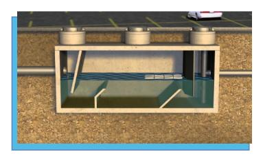
**Underground Vaults and Wells** slow the flow of rainwater runoff and allow pollutants to settle to the bottom to be cleaned out later.
