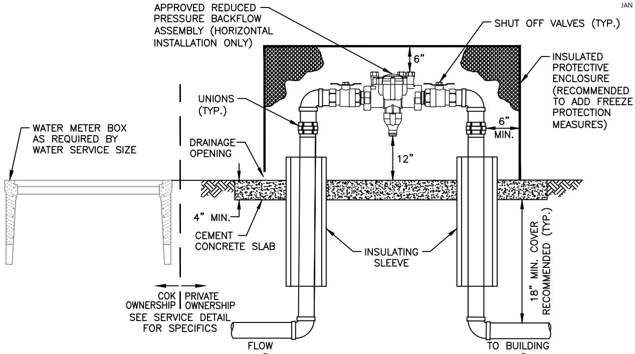
**REDUCED PRESSURE BACKFLOW ASSEMBLY (RPBA)**
