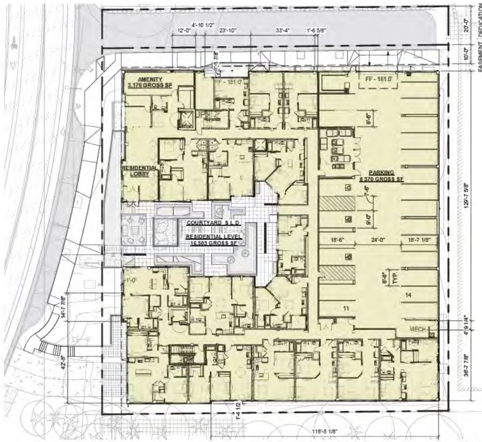
(R1) 2ND FLOOR/UPPER PARKING LEVEL SCALE: 1/32" = 1'-0"
