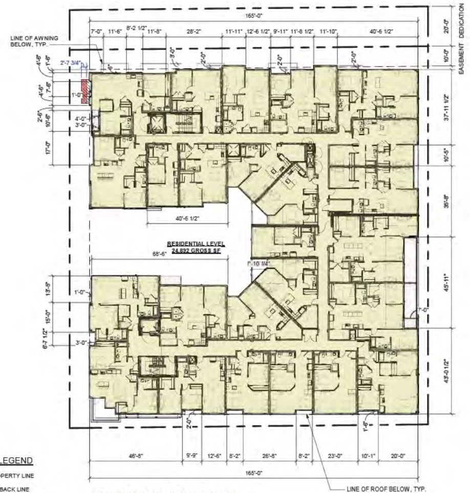
(R2) 3RD FLOOR PLAN SCALE: 1/32" = 1'-0"
