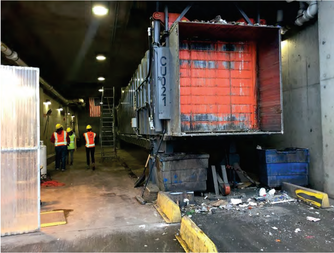
Figure 17 The 85-foot-long SSI 4500SPH compactor. View from bale output end. This mates to hauler trailer.
