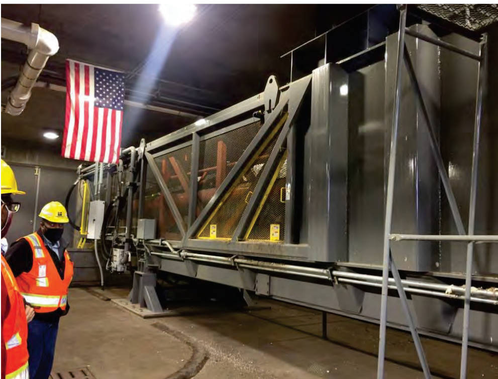
Figure 18 Hydraulic ram end of compactor and waste chute going up to the main floor (left).
