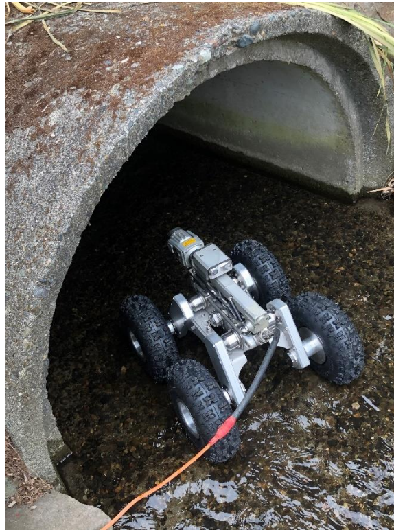
Figure U-15: Remote video rover inspecting a pipe
