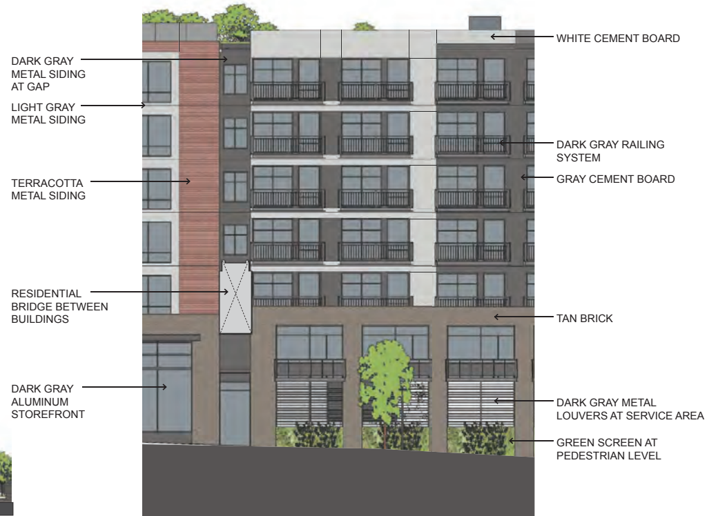
2 ENLARGED NORTH FACADE DETAILING
