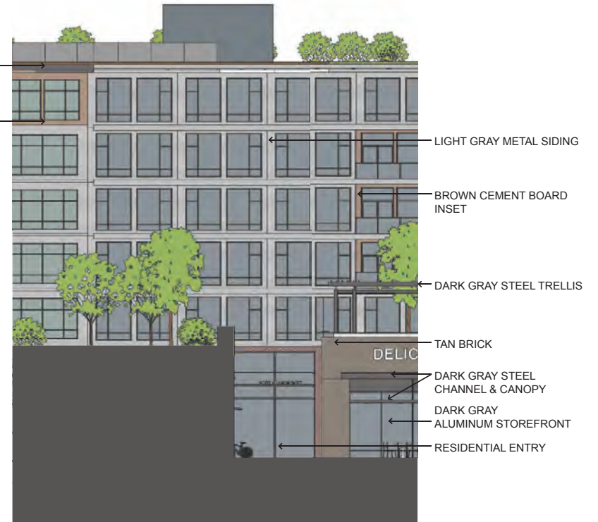
2 ENLARGED EAST FACADE DETAILING
