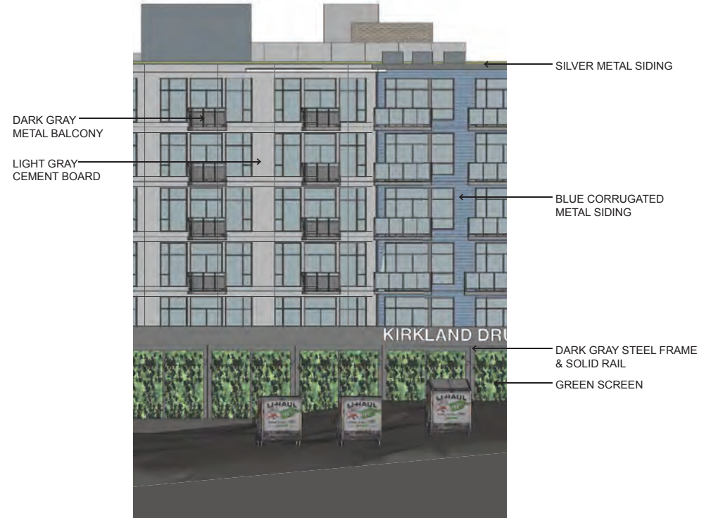
2 ENLARGED WEST FACADE DETAILING
