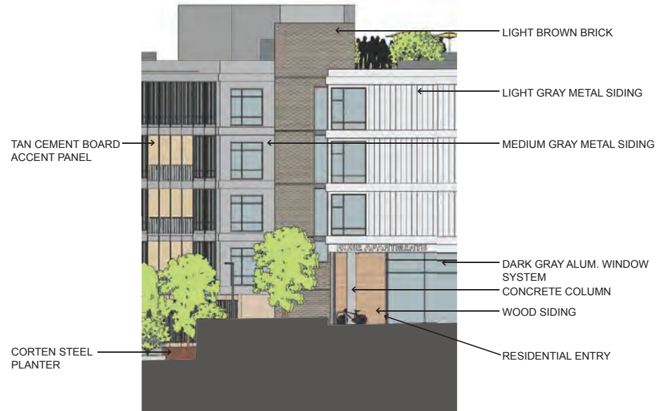
2 ENLARGED SOUTH FACADE DETAILING SCALE: 1/16"=1'-0" @ 11x17
