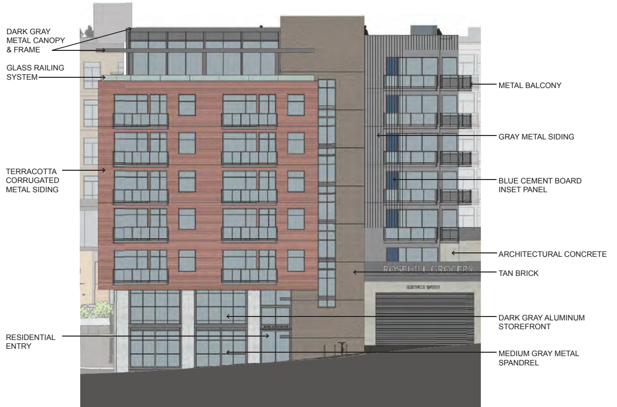
2 ENLARGED WEST FACADE DETAILING
