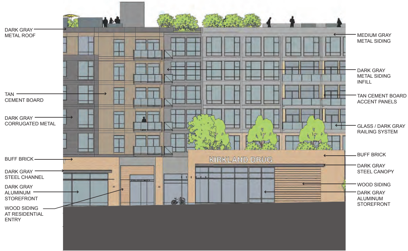
2 ENLARGED WEST FACADE DETAILING
