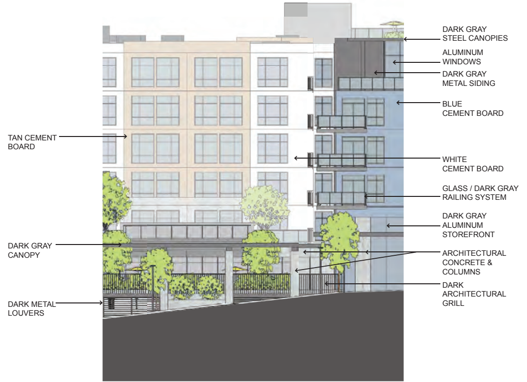
2 ENLARGED SOUTH FACADE DETAILING
