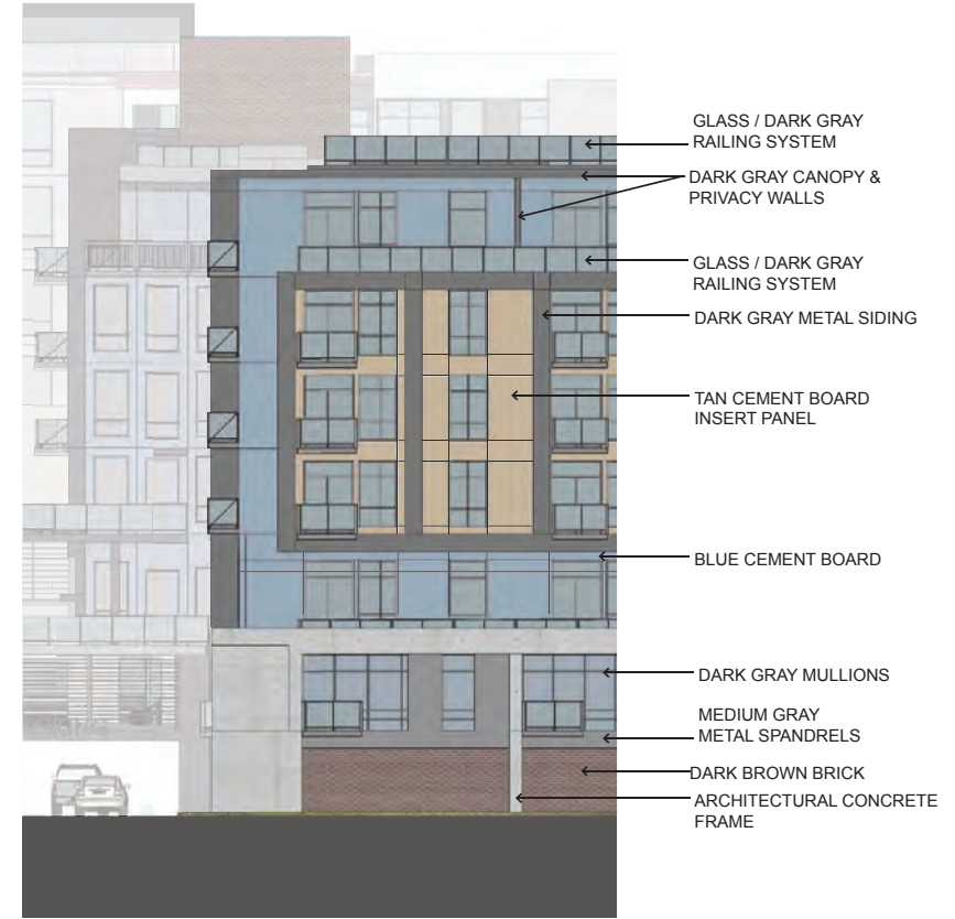
2 ENLARGED NORTH FACADE DETAILING SCALE: 1/16"=1'-0" @ 11x17
