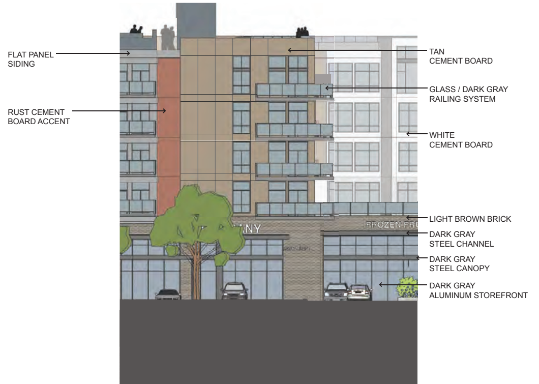
2 ENLARGED SOUTH FACADE DETAILING
