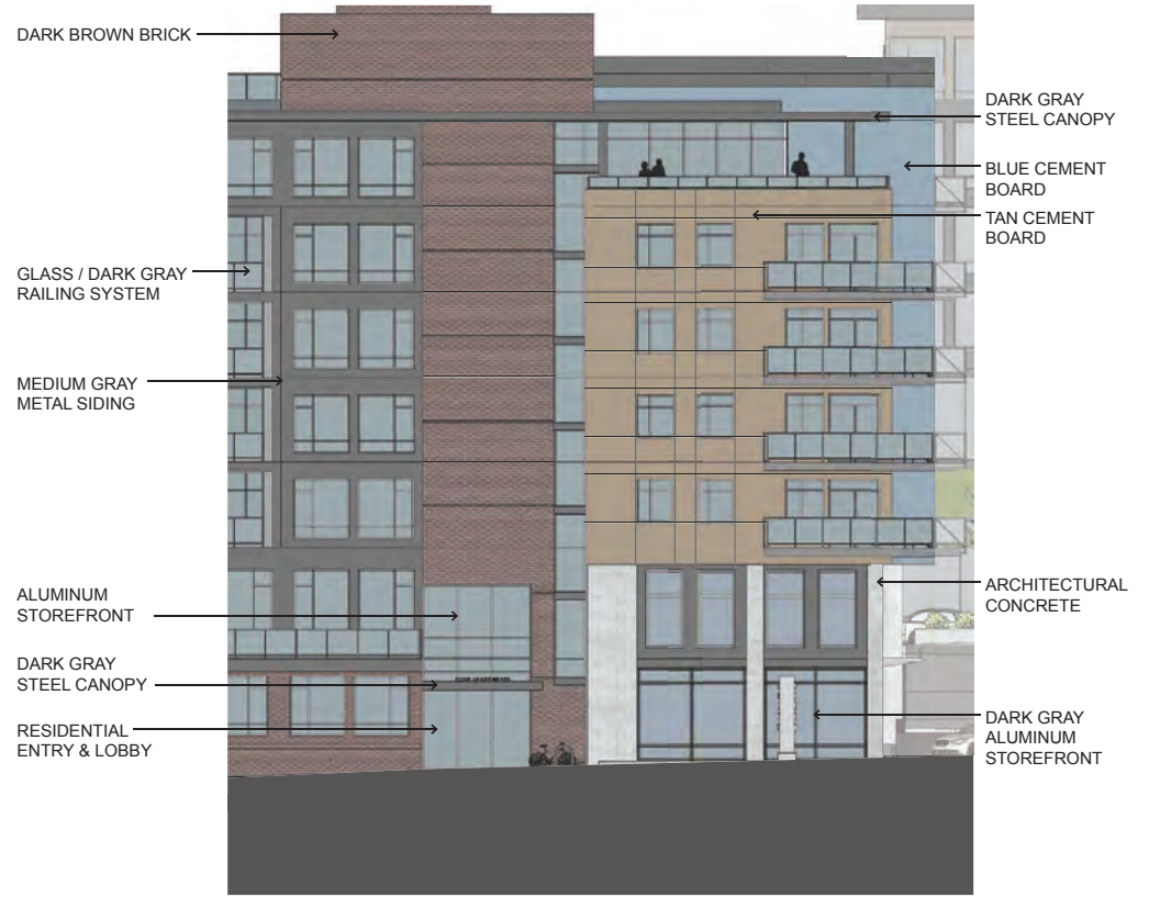
2 ENLARGED WEST FACADE DETAILING
