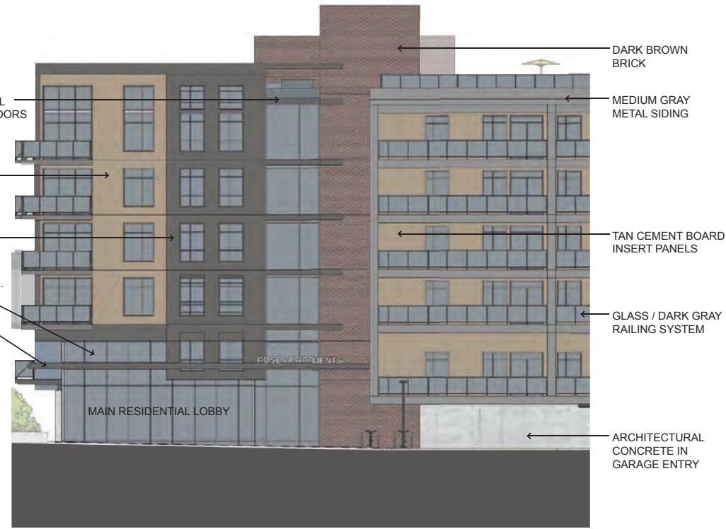
2 ENLARGED EAST FACADE DETAILING
