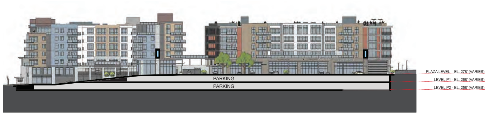
4 EAST-WEST SECTION AT AUTOCOURT LOOKING NORTH
