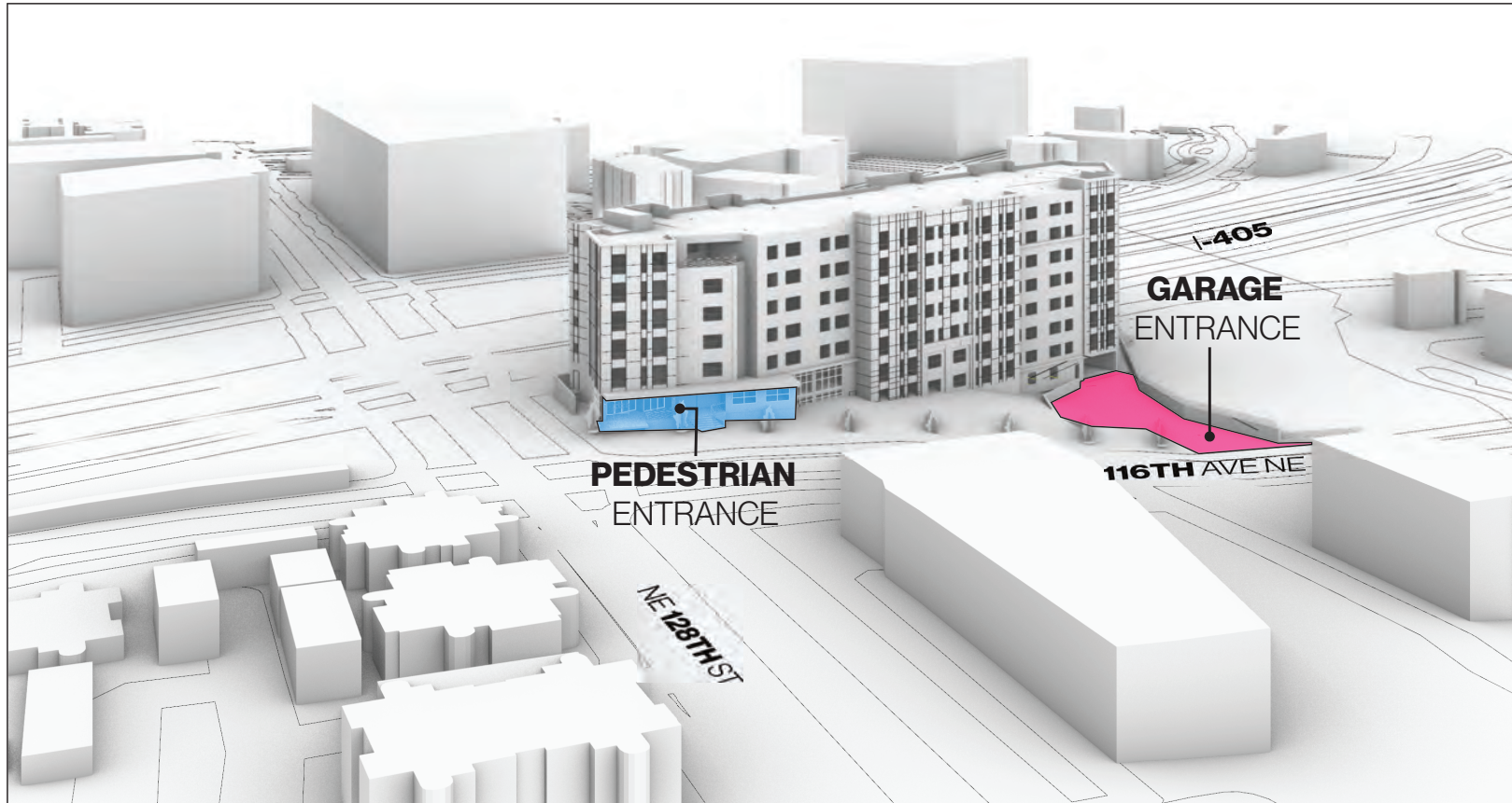
OUR SITE PROPOSES TWO MAIN ENTRANCES, A PEDESTRIAN FOCUSED ENTRANCE TOWARDS THE NORTH WEST CORNER OF THE LOT AND A VEHICULAR ENTRANCE TOWARDS THE SOUTH END. BOTH OF THESE ENTRANCES CAN BE ACCESSED FROM 116TH AVE WHICH HAS LESS TRAFFIC AND MAKES FOR A SAFER TRANSITION ONTO THE PROPERTY.
