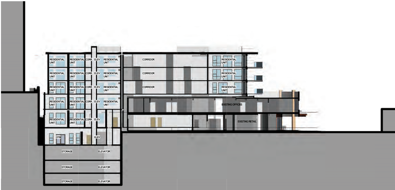
^ SECTION THROUGH NEW CONSTRUCTION AND EXISTING BUILDING
