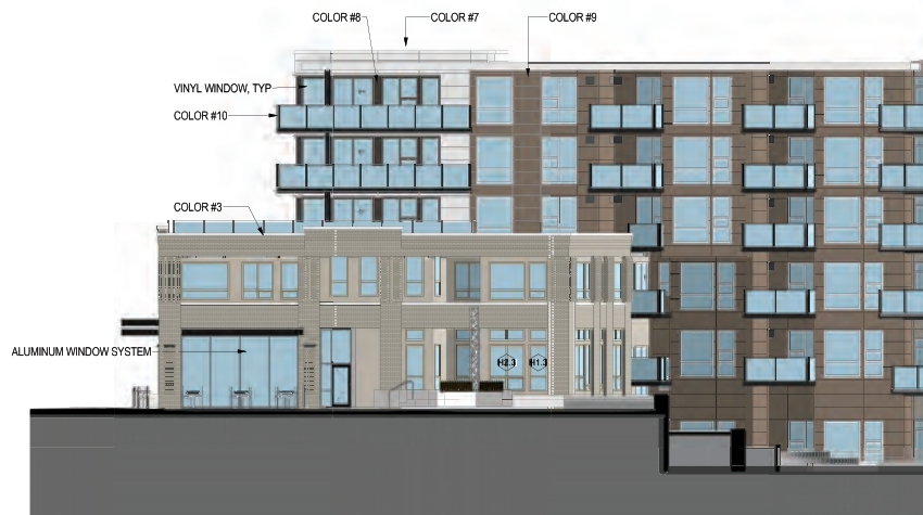
^ COURTYARD SOUTH ELEVATION
