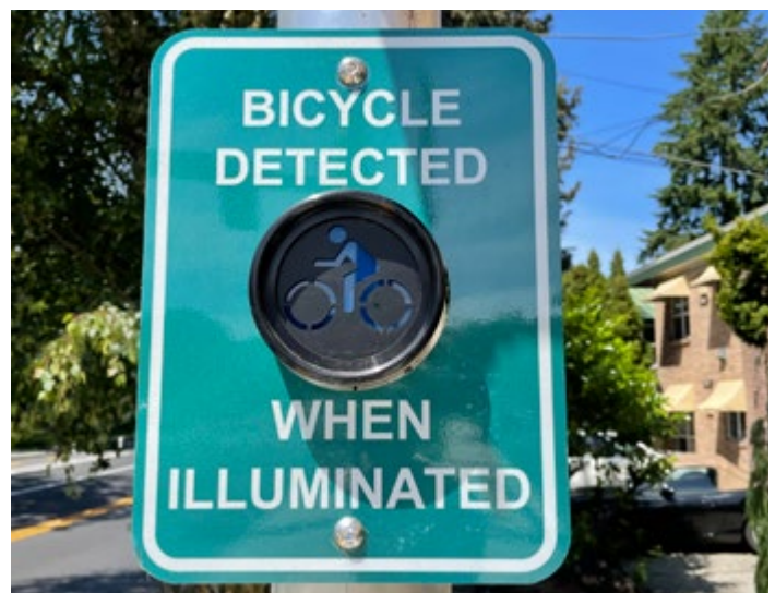
Figure 66. Blue Bike Detection Confirmation Light in Seattle, WA
