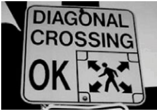
Figure 63. Diagonal Crossing OK sign. Pg 93 of Pedestrian Facilities Users Guide: Providing Safety and Mobility, USDOT Federal Highway Administration Research and Development, Publication number FHWA-RD-01-102, March 2002
