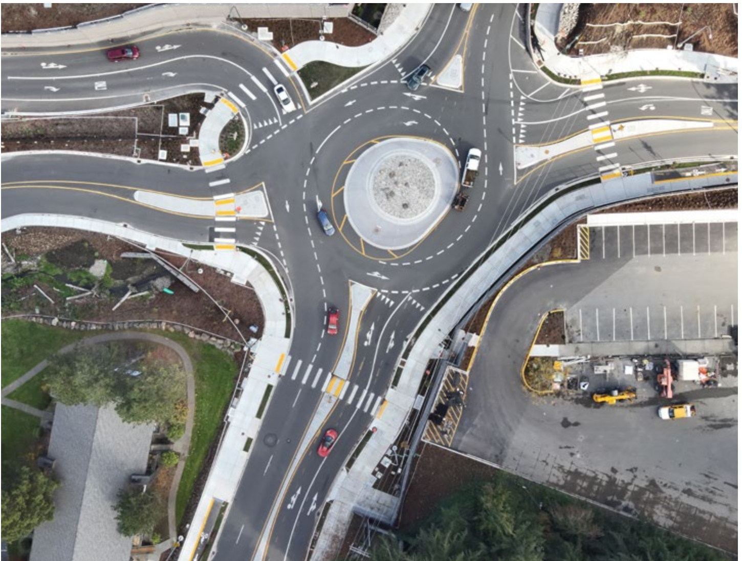
Figure 92. Roundabout with multi-use and bicycle facilities on NE 132nd St at I-405
