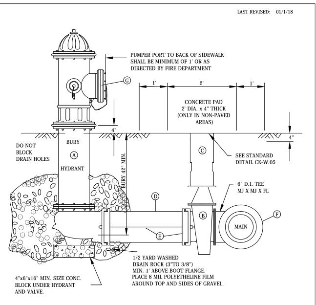
A. 1-5 1/4" M.V.O. HYDRANT WITH 2-2 1/2" N.S.T. AND 1-4" PUMPER, SEATTLE STANDARD.
