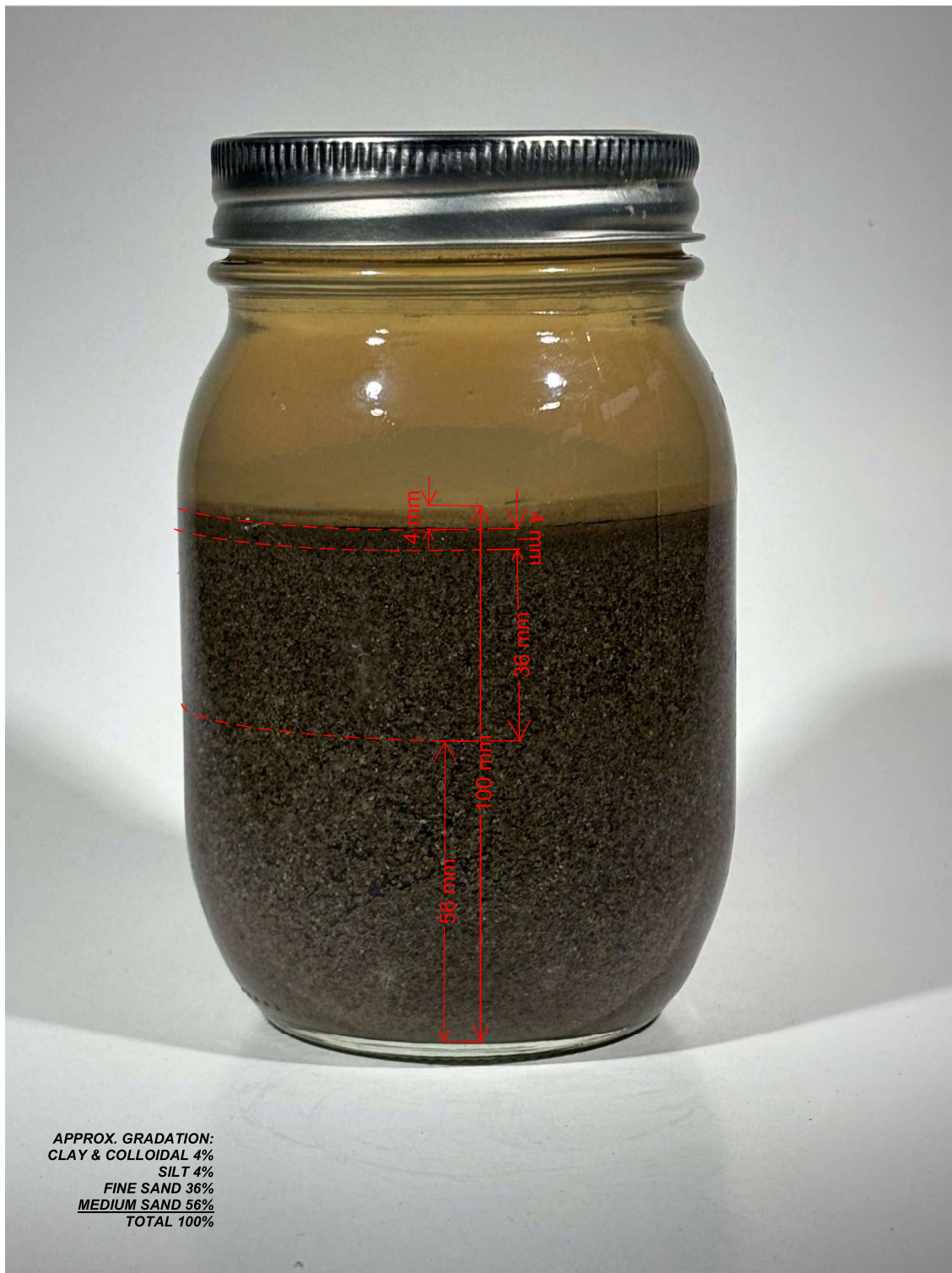
CRESTWOODS PARK FIELD 4 SECTION MATERIALS SETTLEMENT TESTING BASE SAND SAMPLE JUNE 18, 2025
