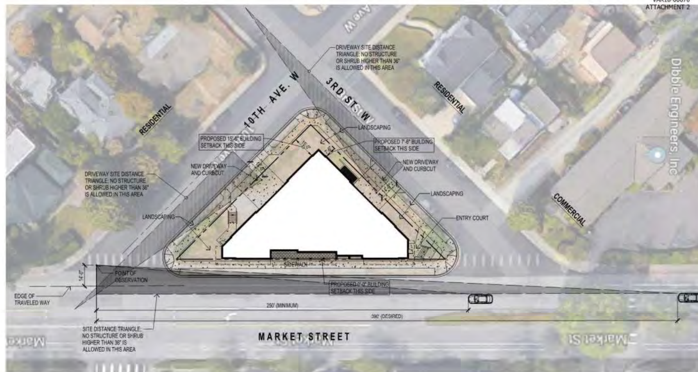
Note: Sight Distance Diagram based on City of Kirkland Policy R-13 - Intersection Sight Distance
