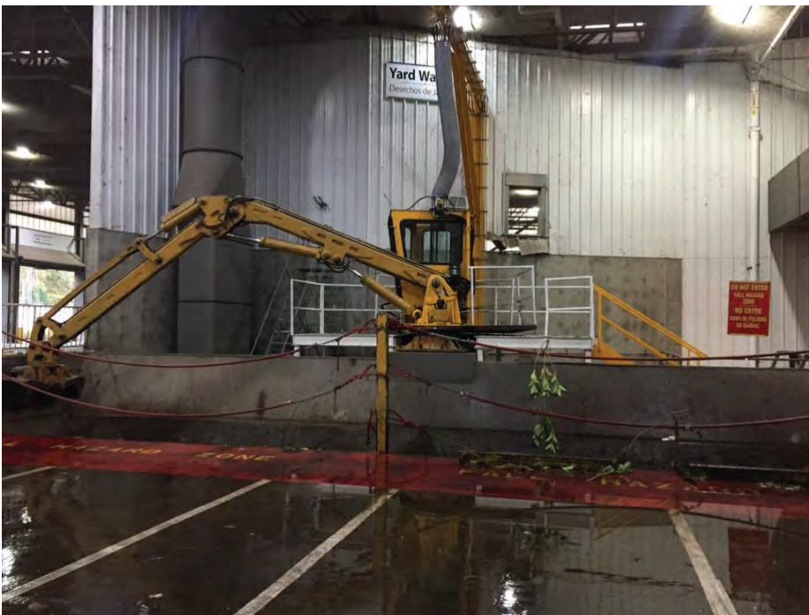
Figure 11 Yard waste drop-off and “old school” Houghton style compactor (yellow).
