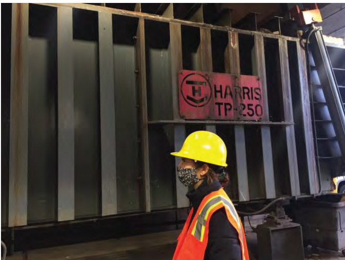
Figure 21 Back-up compactor, the Harris TP-250.
