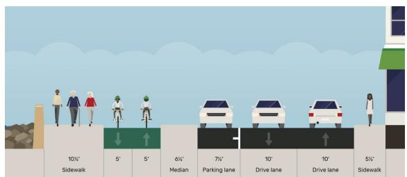
Figure 2 Typical Option 2 Cross Section – Two-Way Protected Bike Lane, <u>West Side</u>
