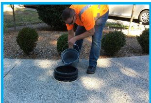
Permeable hard surfaces must pass infiltration tests.
