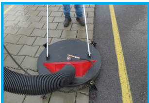
Eductor cleaning head for permeable hard surfaces.
