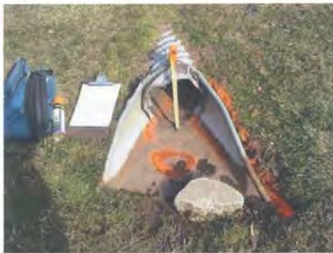
Figure 4.1: Marking outfall deficiencies.
