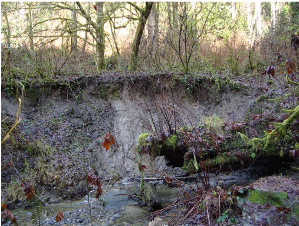
Photo #9. Right bank hillslope failure downstream of Stone Bridge
