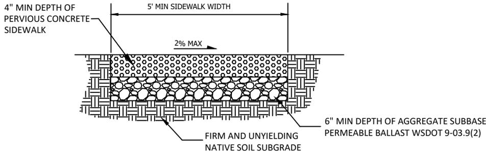
PERVIOUS CONCRETE SIDEWALK SECTION
