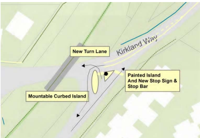
Fig 3. New intersection treatment from 2017 NSP
