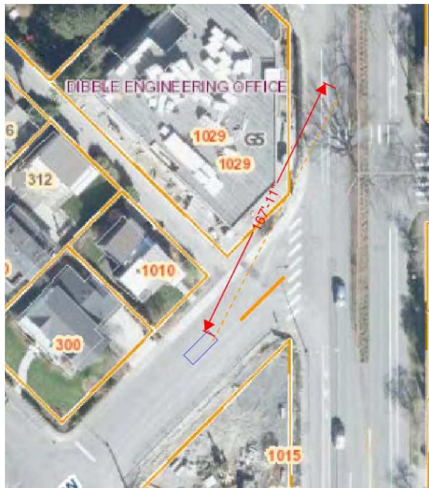
Figure 3. Stopping Sight Distance for The Driveway on 3 rd Street West
