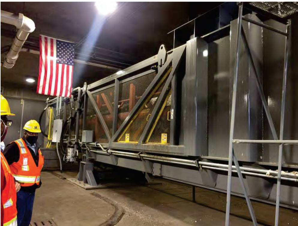
Figure 18 Hydraulic ram end of compactor and waste chute going up to the main floor (left).
