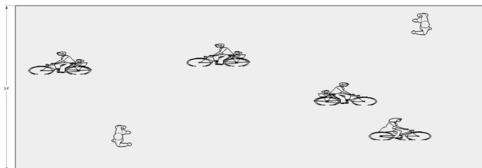
Figure showing 14-ft wide deck with 0.1 persons/m 2 with 67% bicycle traffic
