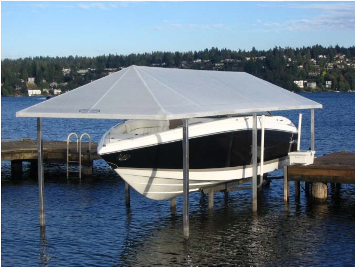
Photograph of boat lift canopy with translucent cover
